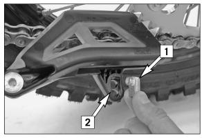
Loosen both screws on the chain guide and pull the chain guide off the swing arm. Turn the chain guide over, press out the retaining nut [1] and insert it in the other hole [2], turning the retaining nut around. Remount the chain guide and tighten the screws.
